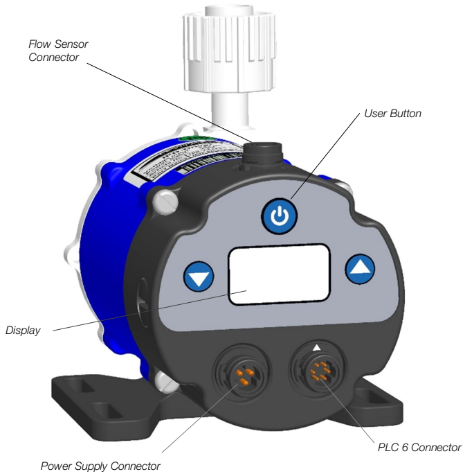
Figure 11: Interface specifications of standard "Stand-Alone" model
